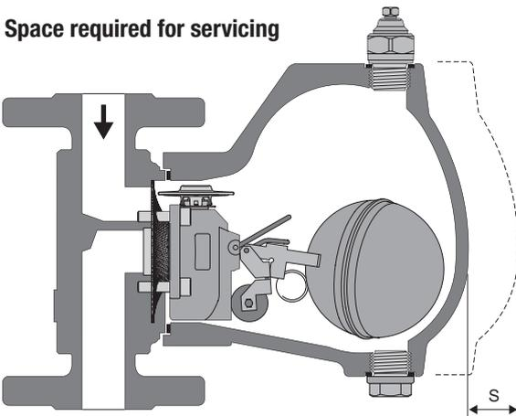
To remove the cover a withdrawal space S of 240/350 mm (depending on size) is required.
