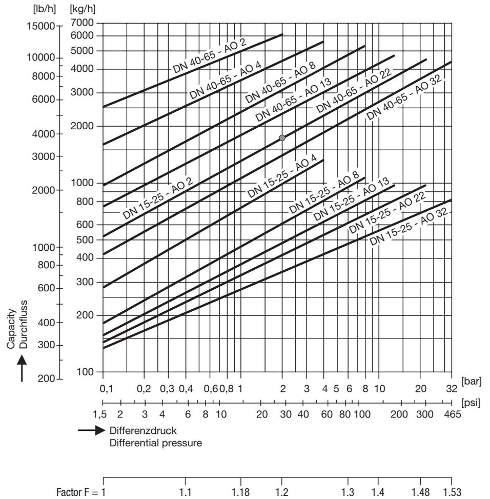
The max. differential pressure  $\Delta$  PMX of the equipment depends on the type of orifice (AO) used.
