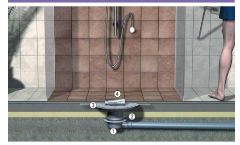
The *Classic* bathroom drain ① is a compact bathroom drain which is available in many versions. It is available both with a vertical and a horizontal outlet ② in the sizes  $\varnothing$  50 and  $\varnothing$  75 mm. There is an adhesive flange ③ available as an option for moisture sealing. The cover is a stainless steel cover in an oval design ④ - but *Classic* bathroom drain can also be combined with any other upper section from the System 100 range.
